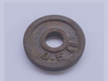
Counterweight It is used to throw tie-rods over the stack. Any object weighting at least 200 g can be used.
